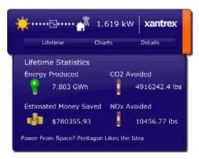
Clicking **Lifetime** displays the Lifetime Statistics drawer, which displays cumulative data for the entire power system.
