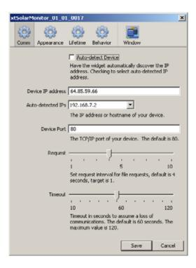
**Auto-detect Device** Select to have the Widget automatically detect the Gateway Device IP address.
