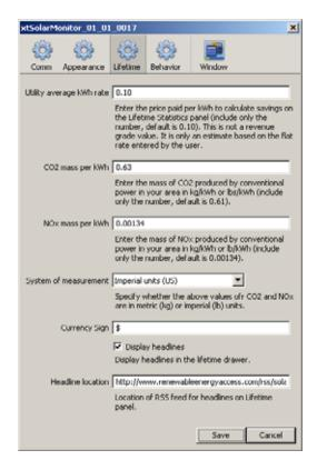
You can configure the Lifetime Statistics display in the Lifetime Preferences. The "Estimated Money Saved" and greenhouse gases (CO2 and NOx) avoided totals displayed in Lifetime Statistics are multiples of the Energy Produced total and the values defined in Lifetime Preferences. In Lifetime Preferences you can also select whether imperial or metric values are displayed in Lifetime Statistics.
