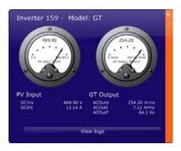
**Important:** The meters range between the minimum and the maximum value of the selected item. When a value is negative (such as current when a device is inverting), the meter indicates a value to the right of the minimum value. Always refer to the numerical values below the meters to determine the direction of the power or current flow.
